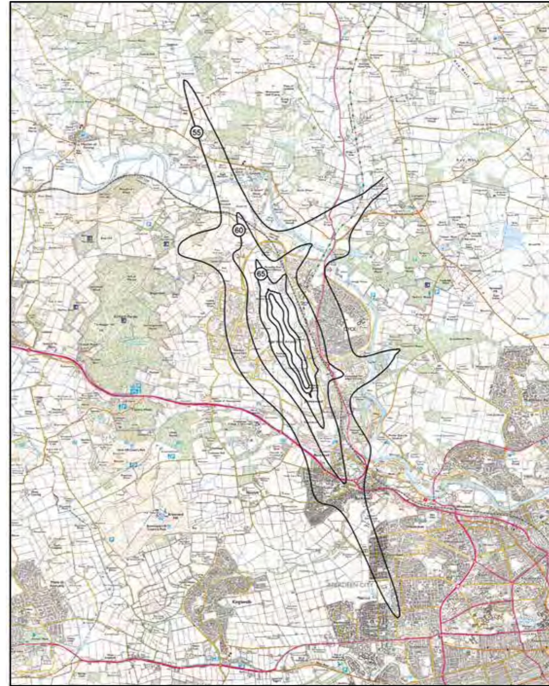
ABERDEEN INTERNATIONAL AIRPORT 2016 Annual Day L Aeq,15hr 55-75 dB(A) Noise Contours (Fixed-Wing + Helicopters) Actual Modal Splits: Fixed-Wing 52% S / 48% N, Helicopters 64% S / 36% N
